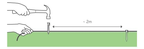
When the edge is flat, use the short distance of the RoboRuler.
