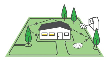
The mower moves randomly within its working area, as defined by the perimeter wire. This kind of random movement provides the perfect cut and ensures complete coverage of your lawn.
