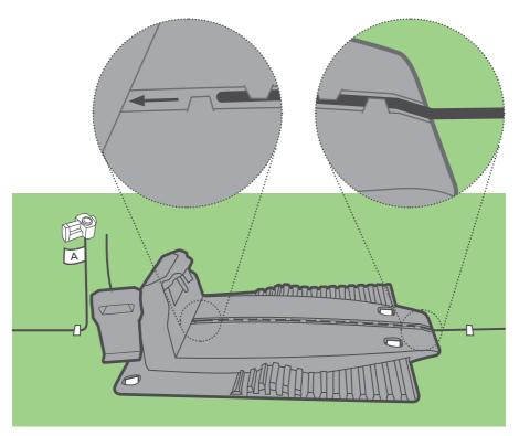
Install the connector to the tip of the wire as described in the drawings. Cut the wire end, close to the connector.
