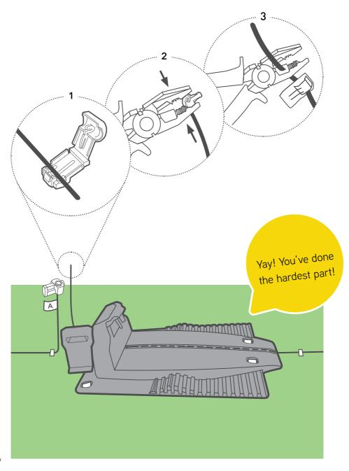
Peg the wire to the ground. Twist and wrap the wires so they could fit nicely in Base Station compartment. Connect the wire end marked with 'A' to the connector marked with A on the back of the Base Station. Connect the other end to the other connector. Tuck the wire in and close the door.
