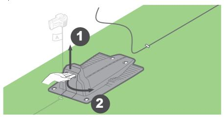
Slide or install the wire through the designated tunnel and pass it through the opening under the charging connectors until it goes out to the back of the Base Station
