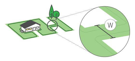
A Narrow Pass connects the Main Zone with a Sub Zone. For passages greater than 2m (6.5 ft), the mower will be able to drive through.
